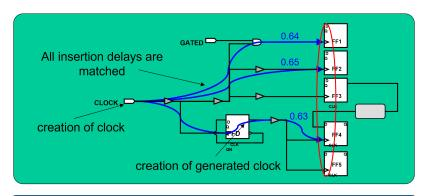
Skew will be balanced globally within each clock domain across all clock-pins for both master and generated clock.
