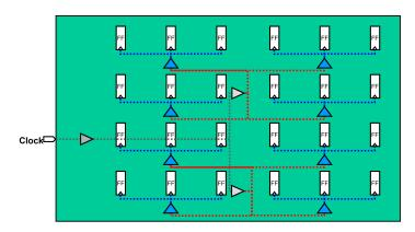
A buffer tree is built to balance the loads and minimize the skew
