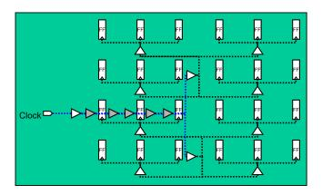
A delay line is added to meet the minimum insertion delay
